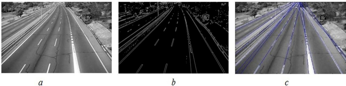
Figure 1. Intermediate results of detection of road region: (a) Background obtained through GMM (b) Result of Canny edge detector (c) Straight lines obtained using Standard Hough Transform
