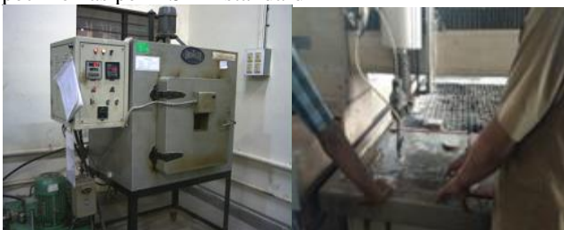
Fig 3: Post curing and specimen preparation
