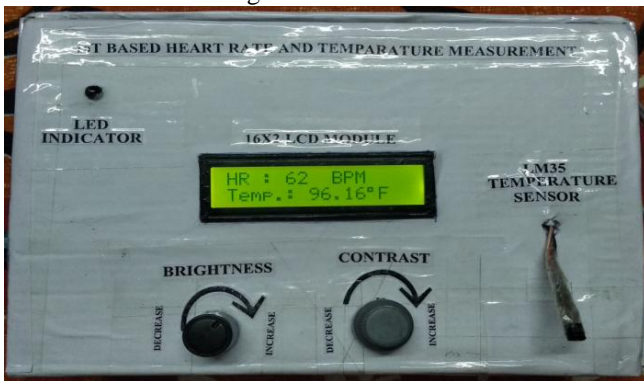
Fig. 8. Result displayed on a 16x2 LCD showing the temperature and heart rate
