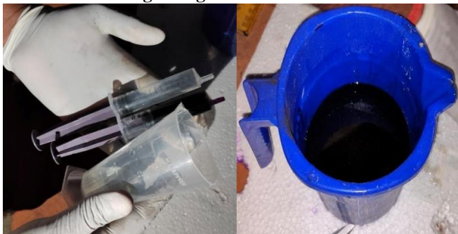
Fig 3: Beaker, syringe and isophthalic resin mixed with hardener and accelerator
