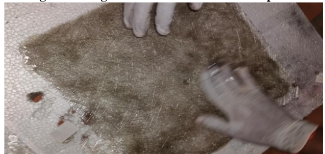
Fig 6: Making of E-Glass fibre reinforced composite
