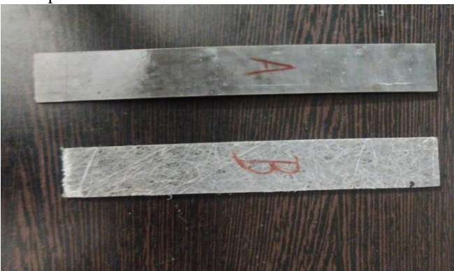
Fig. 7. Test specimen made for Tensile Test
