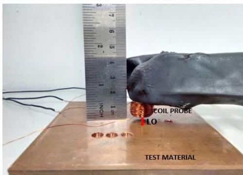
Fig.1. Lift-Off (LO) Measurement
